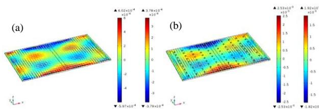
Figure 2. Quasi-thickness shear mode at a resonance frequency of 2 MHz. (a) without circular holes and (b) with circular holes
