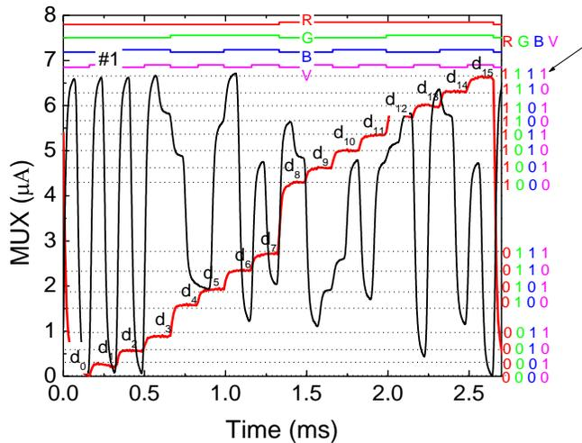
Figure 4. MUX signal of the calibrated cell. On the top the transmitted channels packets [R, G, B, V] are depicted. A received MUX signal is also superimposed to exemplify the decoding process.
