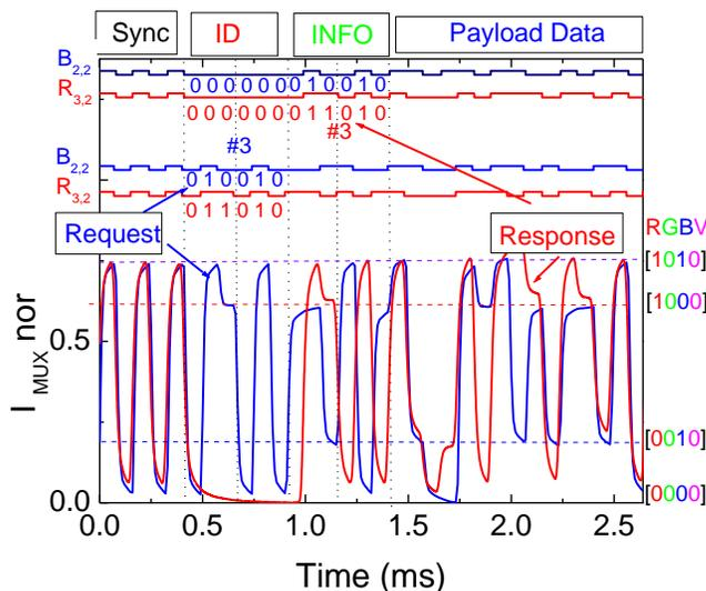
Figure 7. Bidirectional communication: MUX/DEMUX signals assigned to a “request” and a “response” message. On the top the transmitted channels packets  $[X_{i,j}]$  are decoded.
