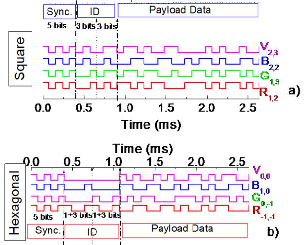
Figure 3. Data frame structure. Representation one encoded message, in a time slot from the array in the network: a) Square topology;  $R_{1,2}$ ;  $G_{1,3}$ ;  $B_{2,2}$  and  $V_{2,3}$  are the transmitted node packet. B) Hexagonal topology;  $R_{-1,-1}$ ;  $G_{0,-1}$ ;  $B_{1,0}$  and  $V_{0,0}$  are the transmitted node packet.
