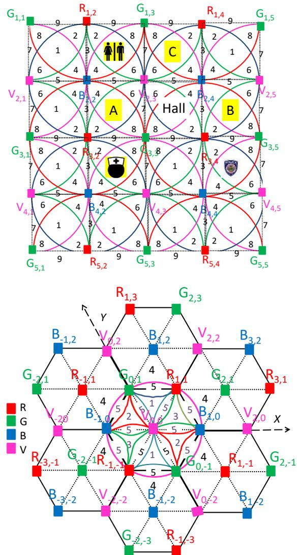
Figure 2. Illustration of the optical scenarios (RGBV >modulated LEDs spots). Cellular topologies: a) Clusters of cells in square topology . b) Clusters of cell in hexagonal topology.
