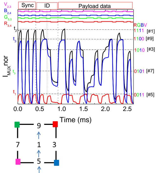
Figure 5. Fine-grained indoor localization and navigation in successive instants ( $t_1$ ,  $t_2$  and  $t_3$ ): MUX/DEMUX signals in a point-to-point path across the main hall ( $\#5 > \#1 > \#9$ ) at the. On the top the complete transmitted channels packets [R, G, B, V] are decoded.
