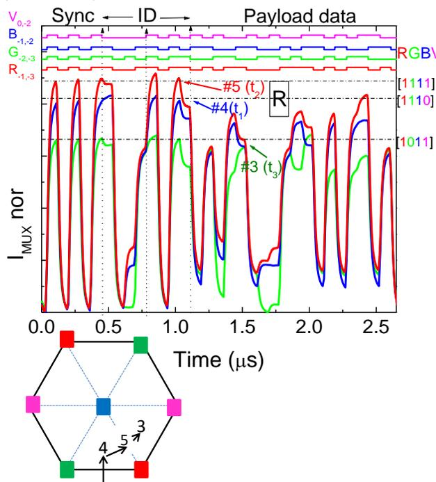
Figure 6 Fine-grained indoor localization and navigation in successive instants  $t_1$ ,  $t_2$  and  $t_3$ . Signal acquisition through the restaurants area (R). On the top the transmitted channels packets are decoded [R, G, B, V].
