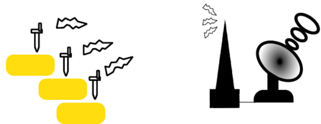
Figure 2. Ground communication network is formed by probes installed in the silos, a hub (data concentrator) coupled to a ground station that transmits the signal to the satellite
