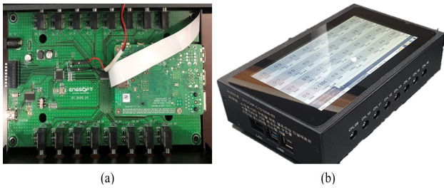
Figure 5. Data logger prototype: (a) Inside circuit, (b) External geometry.
