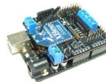
Figure 7. The control board with an xBee-shield attached.
