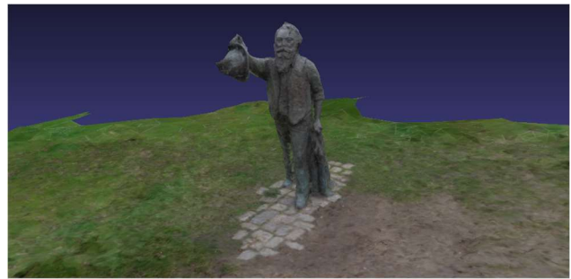
Figure 3. Screenshot of a 3D object reconstructed with NOC3D from 225 images automatically extracted from semantically annotated videos. The blue background is rendered by the 3D object viewer.
