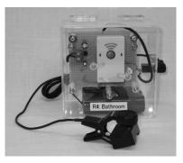
Figure 2. Prototype of the water flow sensor which consists of a vibration microphone, a sound-activated switch (the upper image), an active RFID tag (the lower image), and a battery.
