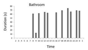
Figure 7. Distribution of the duration of water flow at the toilet's flush tank.
