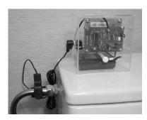
Figure 3. Vibration microphone clipped to the water pipe to the flush tank of a toilet.
