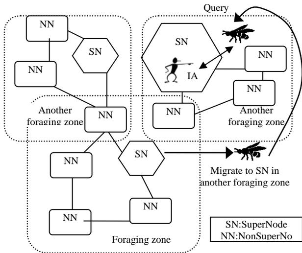
Figure 2. The activities of long distance bee agents to locate a resource. They communicate with super nodes.
