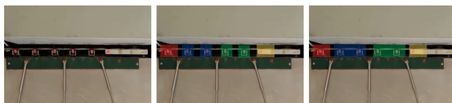
Figure 5: (a) Left: After step 7 of the calibration algorithm. The locations (red points) of the weighting springs along the conveyor belt are acquired. (b) Middle: During step 8 of the calibration algorithm where each point is enclosed into a polygon. (c) Right: Towards the end of step 8, where the polygons of weight springs that are responsible for the same egg size are merged and the zones are finally formed.
