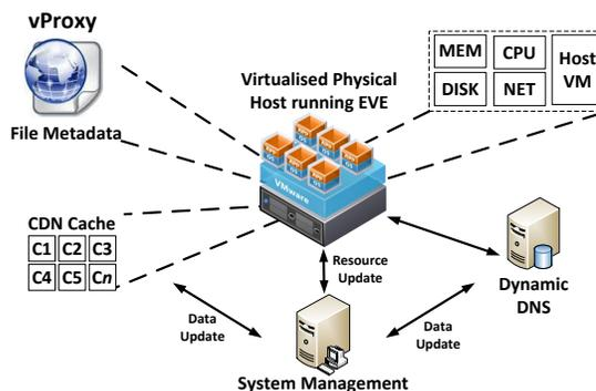
Fig. 3: Components of an Elastic Video Endpoint
