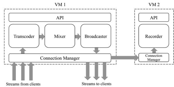
Fig. 1: Example of two MCUs performing different tasks.
