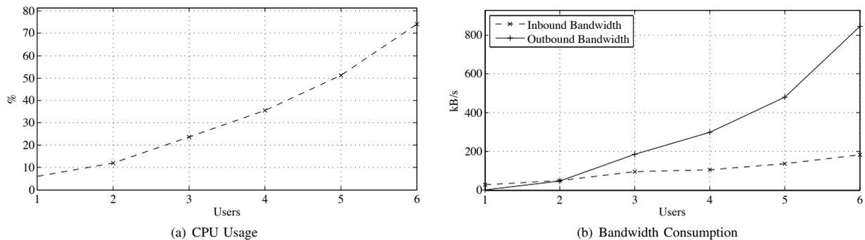
Fig. 4: Use of resources in the MCU when the number of users increases in a videoconference
