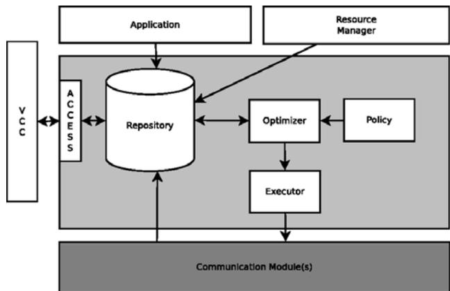
Figure 2. Castalia cognitive radio module (CRModule) internals
