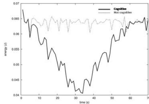
Figure 8. Power consumption for the Cognitive algorithm and 802.15.4 (Scenario 3)
