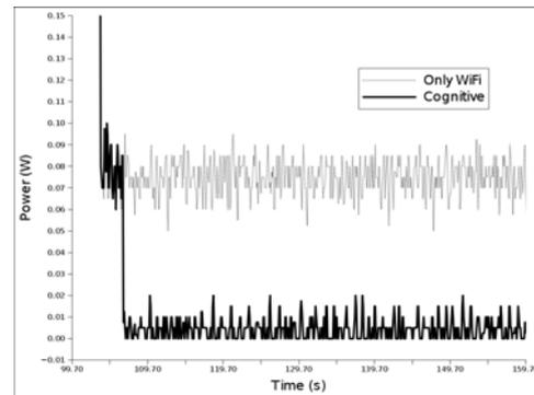
Figure 5. Detail of power consumption for the Cognitive algorithm and WiFi
