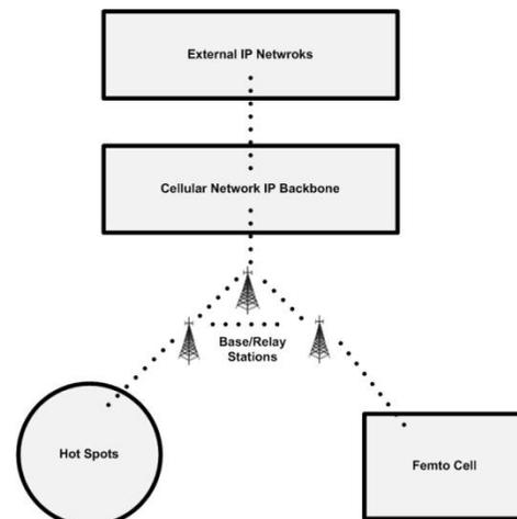
Fig. 4. Basic Architecture of Cellular Network
