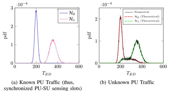
Fig. 2. Pdfs of the ED decision statistic: Parameters:  $N = 50$ ,  $K = 4$ ,  $M_f = 150$ ,  $M_b = 150$  and SNR = -6 dB
