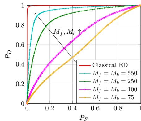
Fig. 3. ROC performance for the considered scenario, Parameters:  $N = 100$ ,  $K = 4$  and SNR = -6 dB
