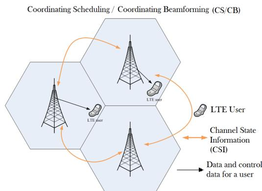
Figure 3. coordinated scheduling / coordinated beam-forming (CS/CB)
