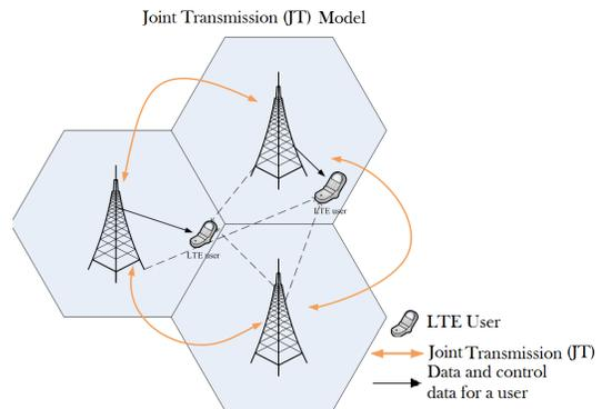
Figure 4. Joint Transmission (JT)
