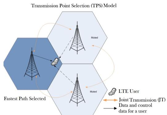
Figure 5. Transmission Point Selection (TPS)
