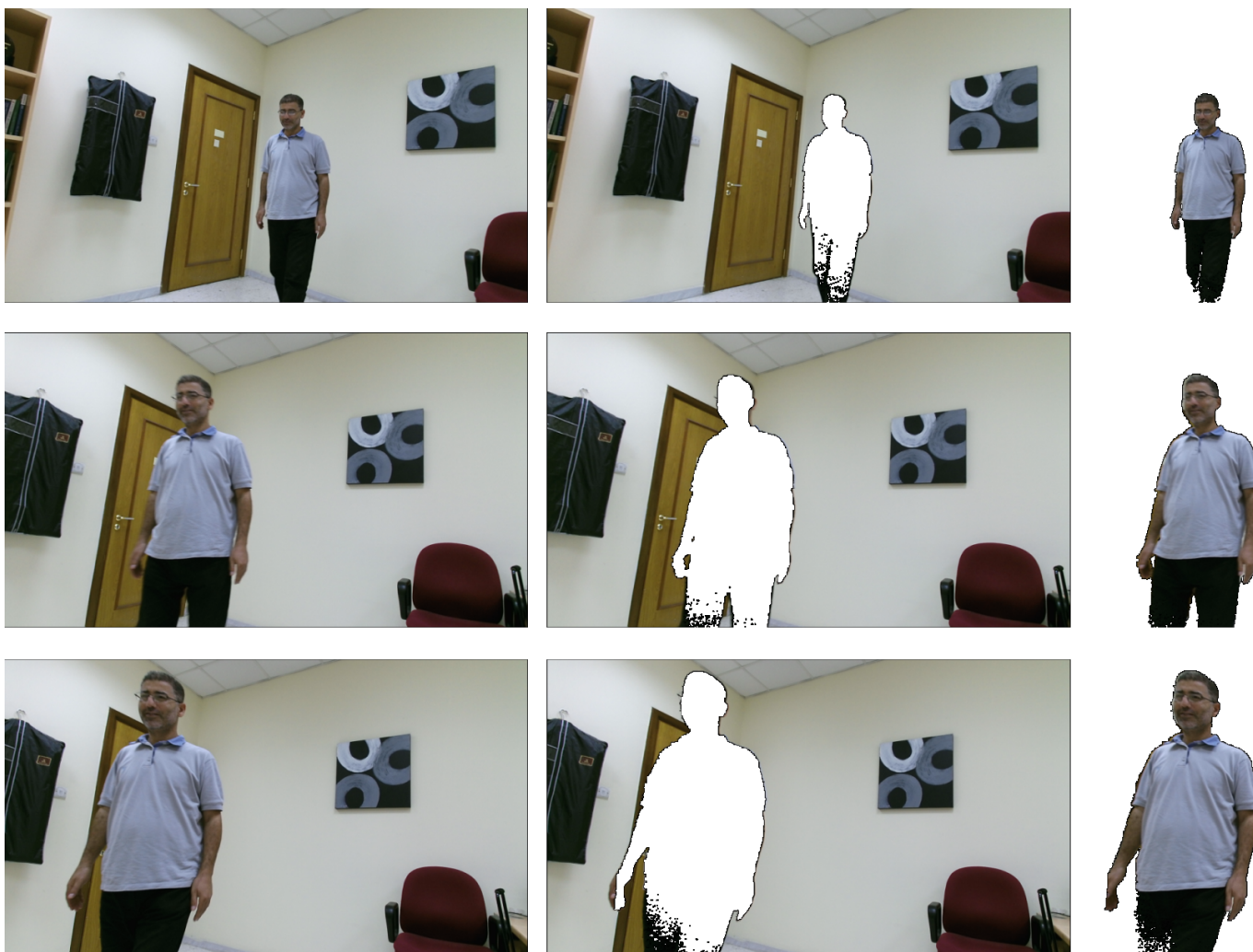
Figure 4. (left) the original RGB frame, (middle) segmented background, and (right) segmented foreground. The motion of the object and the camera is evident from these images.
