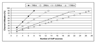
Figure 13. Channel utilization vs. number of VoIP streams for G.711 voice codec (64kbit/s).
