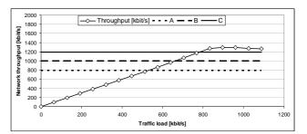
Figure 7. Network throughput vs. traffic load (where triggering levels are denoted as follows: A - switch from AM Mode to std., B - switch from std. to AM Mode, C - switch to Closed Network Mode).
