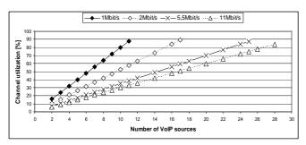
Figure 14. Channel utilization vs. number of VoIP streams for G.726 voice codec (32kbit/s).
