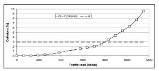
Figure 8. Collisions vs. traffic load (where A denotes the critical level of collisions).
