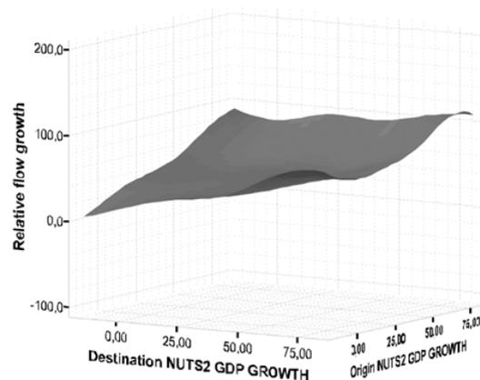
Figure 2. Smoothing interpolation of 3D Scatterplot between Origin and Destination GDP growth and freight flow variation.
