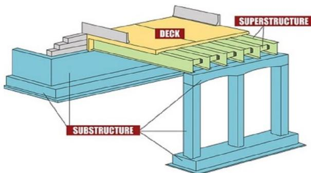
Figure 3: Structural elements of a bridge [21].
