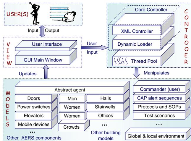
Figure 4. Structure and major components of AERS-SF
