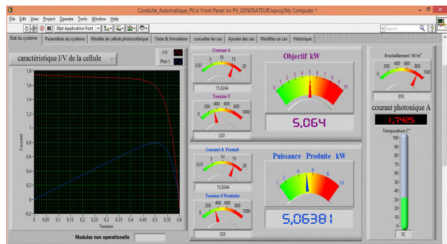
Figure 7. Dashboard of the PV system
