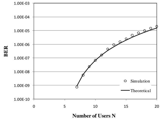
Figure 5. BER versus the number of users N for theoretical and simulation (F=127, k=3).
