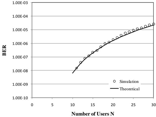
Figure 4. BER versus the number of users N for theoretical and simulation (F=464, k=4).
