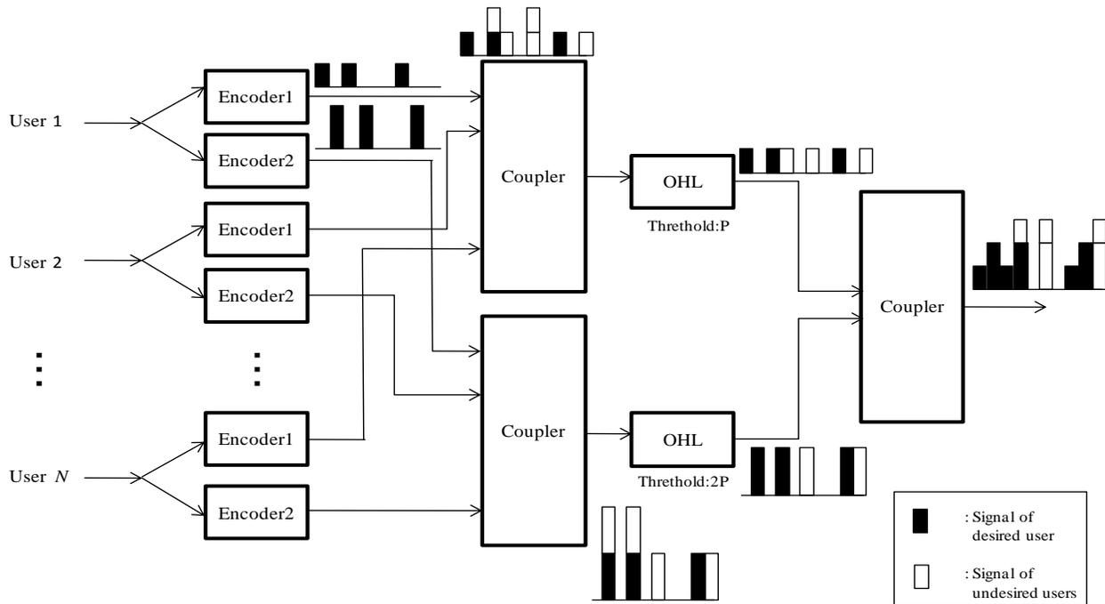
Figure 1. Block diagram of the transmitter of the proposed system.
