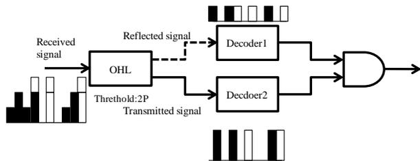
Figure 2. Block diagram of the receiver of the proposed system.
