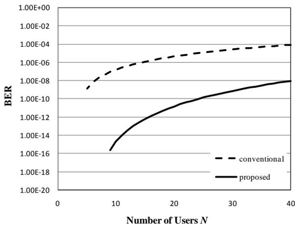
Figure 6. BER versus the number of users N for conventional optical CDMA and our proposed system (F=620, k=4).
