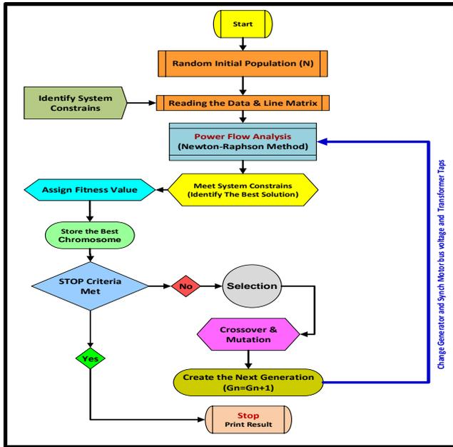
Figure 1. The GA algorithm evolution process flowchart
