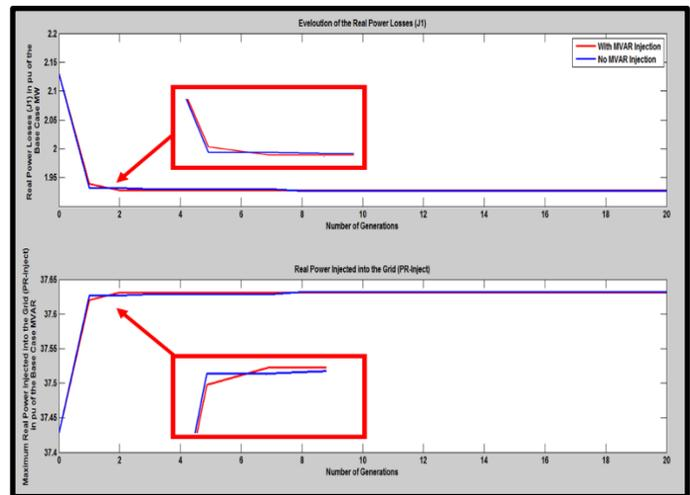
Figure 3.  $J_1$  and  $PR_{Inject}$  value convergent for 10 generations
