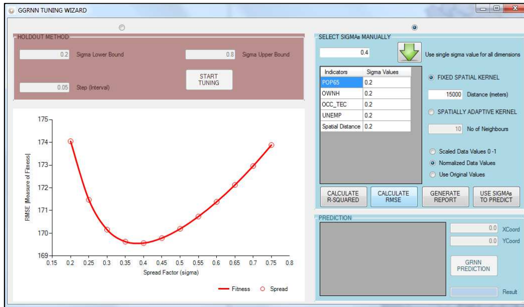
Figure 4. GRNN sigma tuning and prediction tool
