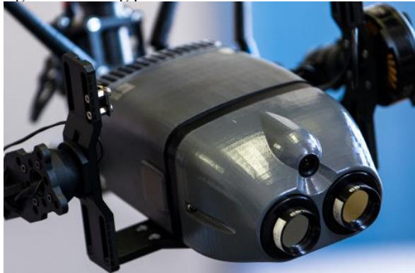
Figure 3: A closer look at the NIR sensor with two CMOS optical sensors placed side by side and furnished with ultra-narrow filters.
