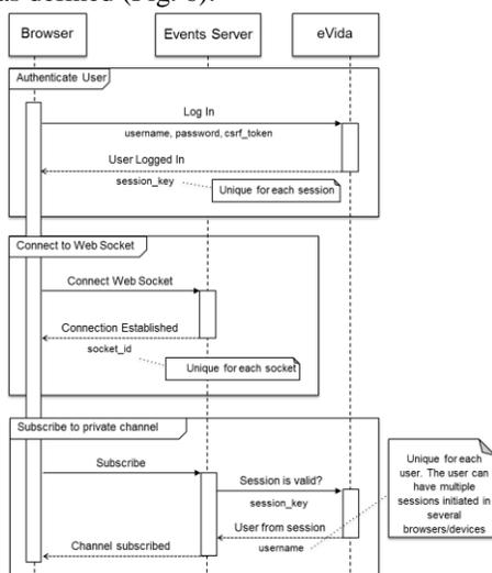
Figure 6. Protection mechanism for private communication channels.
