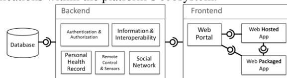
Figure 1. The platform’s high-level architecture.
