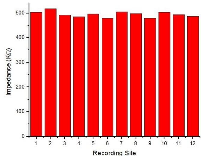
Figure 3. Impedance of the recording sites at 1 KHz.
