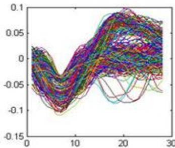
Figure 4. Neural recordings from six recording sites from the developed neural probe array.
