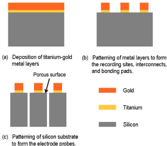
Figure 1. Schematic illustration of the steps involved in the fabrication process of the neural probe array (The Figure is not to scale).
