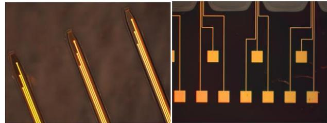
Figure 2. Images of the fabricated porous neural probe array. (a) Close-up image of the probe probes with recording sites; (b) Bonding pads.
