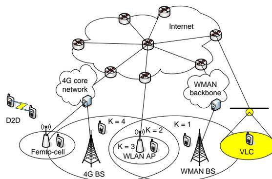
Figure 1. Illustration of a heterogeneous wireless network [30].
