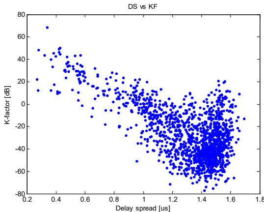
Figure 7. The Correlation for DS vs KF
