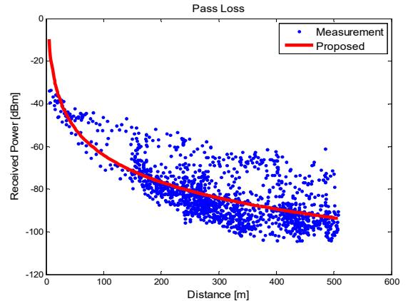
Figure 3. Path loss according to the distance
