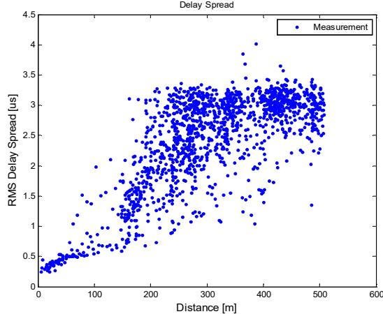
Figure 4. RMS Delay Spread according to the distance
