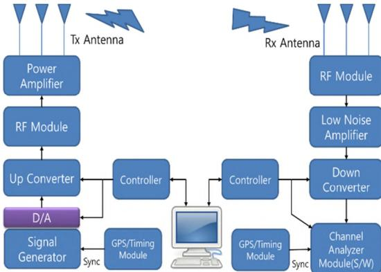
Figure 1. Measurement system configuration
