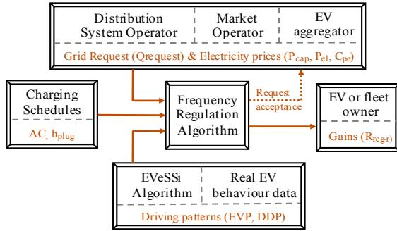
Figure 1. Frequency regulation algorithm interactions
