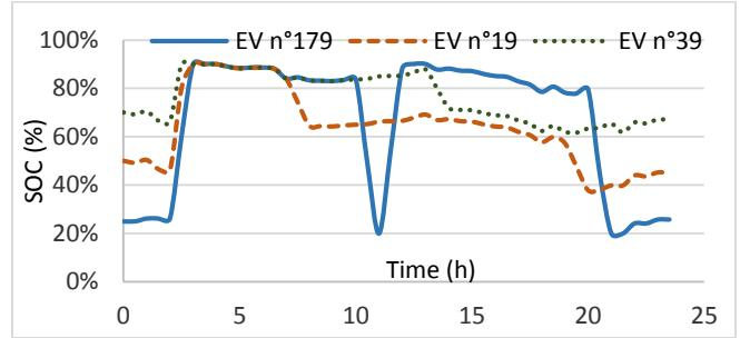
Figure 3. EVs batteries State of Charge (SOC) variation, 2015/02/25
