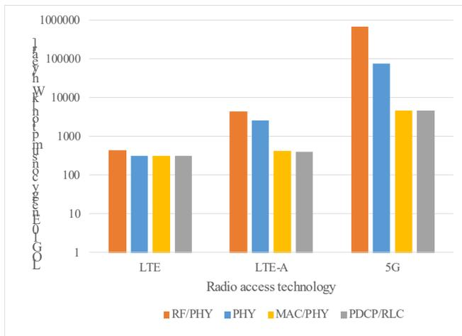
Figure 6. Energy consumption by radio access technology.
