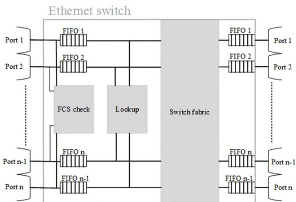
Figure 3. The construction of an Ethernet switch.
