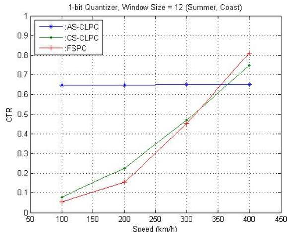
Figure 3. CTR vs. UAV1 speed at 1-bit Quantizer, window size 12 (Summer, Coast)
