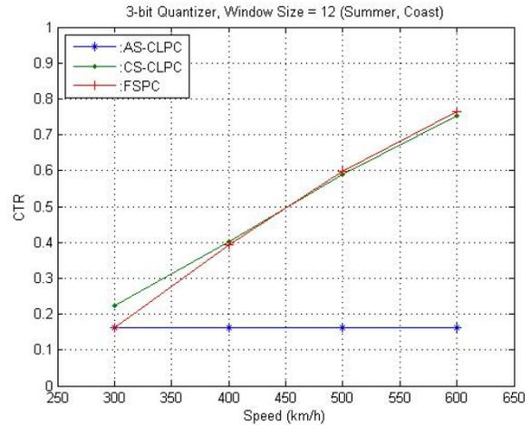
Figure 7. CTR vs. UAV1 speed at 3-bit Quantizer, window size 12 (Summer, Coast)
