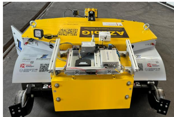
Figure 11 ASV integrated hardware for autonomous driving
