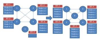
Figure 3. Routing algorithm based on the complete connection among nodes
