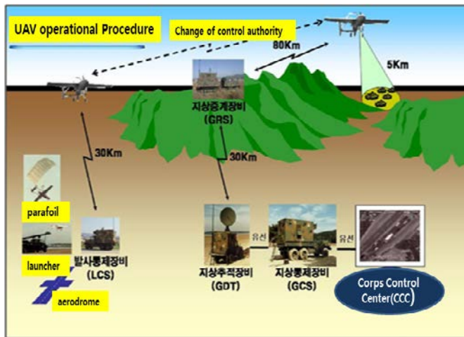
Figure 3. Operations of Real UAV System.
