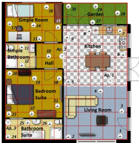
Figure 2. The deployment of the sensor nodes and access points over the house scenario.
