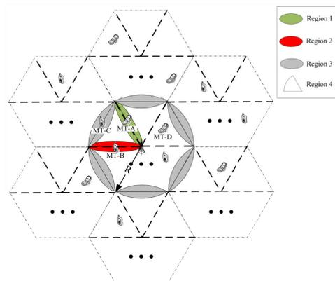
Figure 1. Generalized topology of a sector-based cellular network
