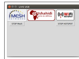
Figure 7. Server LiveUSB GUI for starting/stopping various services like Mesh Networking, Ushahidi and Hotspot.
