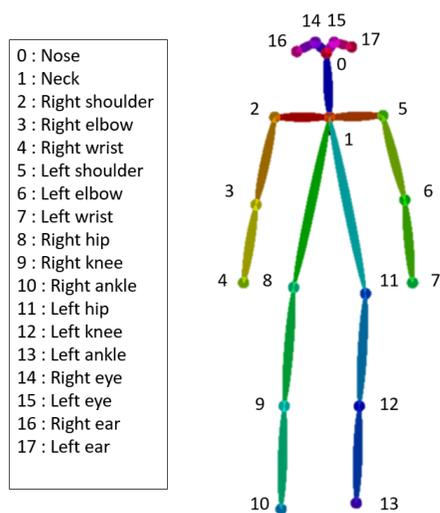
Figure 2. The 18 body joints generated from OpenPose.
