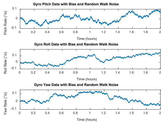
Figure 7. Noisy IMU data - angular velocity
