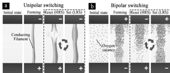
Figure 1. Dynamic growth and formation/rupture processes of filament-type resistive switching mechanism in unipolar (a) and bipolar switching (b) modes [3].
