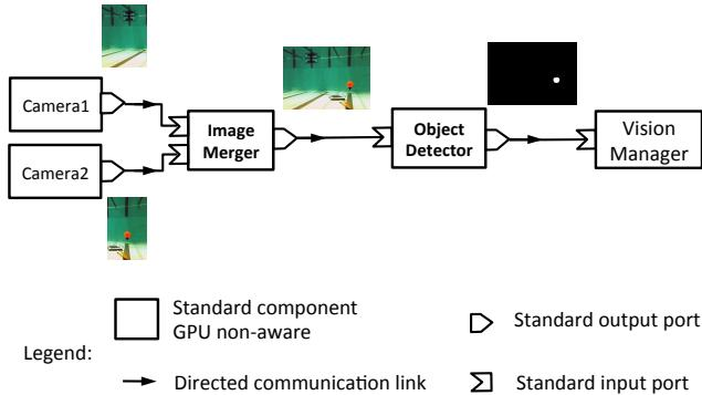
Figure 1. The abstract software architecture of the vision system
