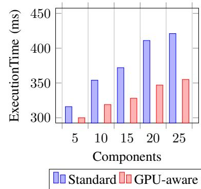
Figure 9. Execution times of two types of systems when processing an image with  $1152 \times 864$  pixels
