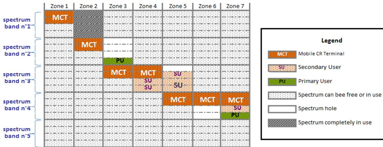
Figure 3. Example of dynamic spectrum distribution
