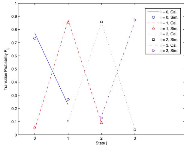
Figure 5. Comparison of transition probabilities for the MIMO-GMD channel capacity (with  $f_D = 30\text{Hz}$ ,  $\tau = 0.001\text{sec}$  and  $\gamma = 10\text{dB}$ ) in a (2,2) system obtained from calculations and simulations.
