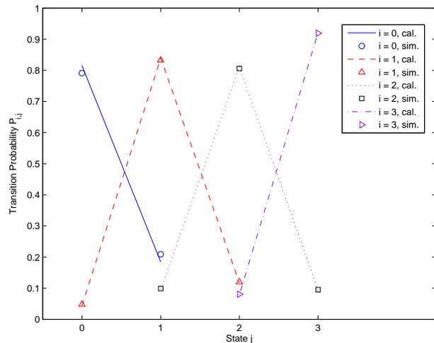
Figure 4. Comparison of transition probabilities for the eigenmodes geometric mean (with  $f_D = 30\text{Hz}$ ,  $\tau = 0.001\text{sec}$ ) in a (2,4) MIMO system obtained from calculations and simulations.
