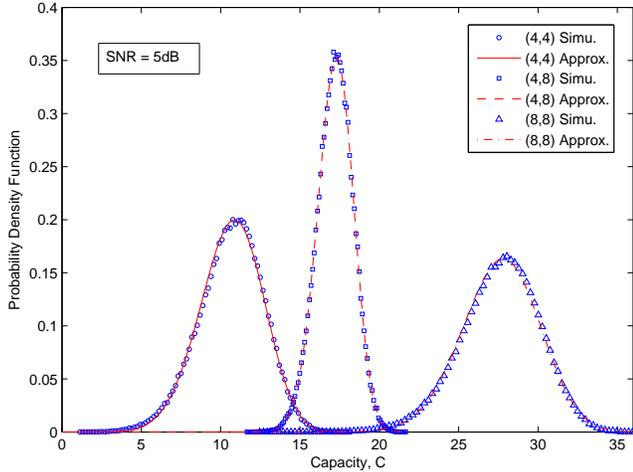
Figure 3. Comparison between simulation and calculation results for distributions of system capacity using GMD in (4,4), (4,8) and (8,8) MIMO Rayleigh fading channels. Assuming  $\gamma = 5dB$ .
