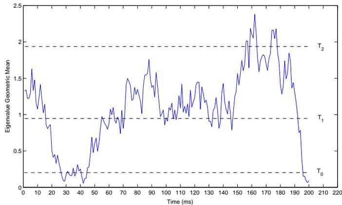
Figure 1. An example of a Markov state quantization. The time-varying eigenmodes geometric mean process in a (2,2) MIMO channel is partitioned into four states using three threshold levels:  $T_0$ ,  $T_1$  and  $T_2$ .
