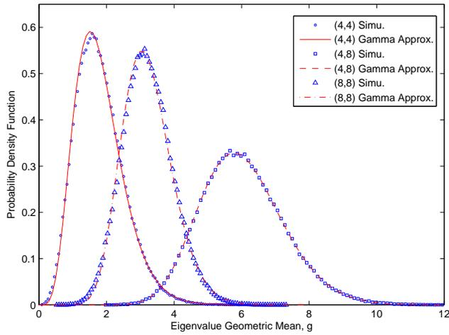
Figure 2. Comparison between simulation and Gamma approximation results for distributions of eigenvalue geometric mean (sub-channel power gain) in (4,4), (4,8) and (8,8) MIMO Rayleigh fading channels.
