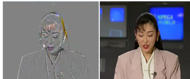
(a) No CLD, frame 59, PSNR= 12.76dB (b) Basic CLD, frame 59, PSNR= 28.52dB Figure 5. Subjective evaluation of the low motion video (Akiyo)
