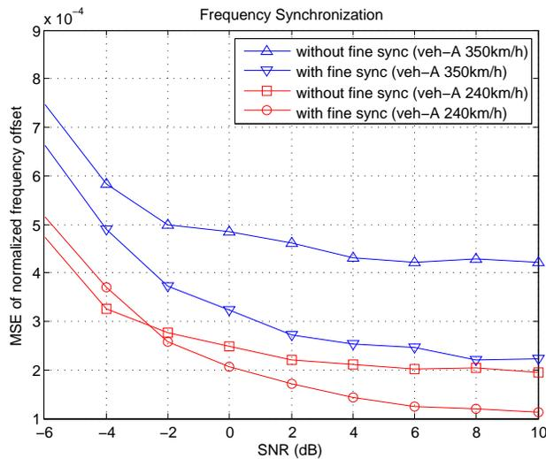
Figure 4. Mean Squared Error of frequency synchronization
