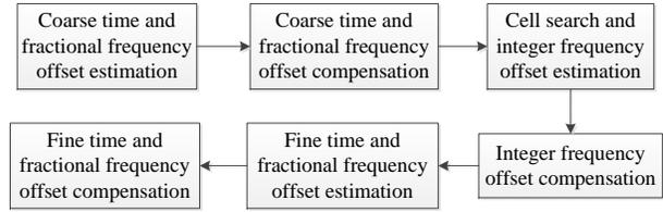
Figure 2. Proposed synchronization process
