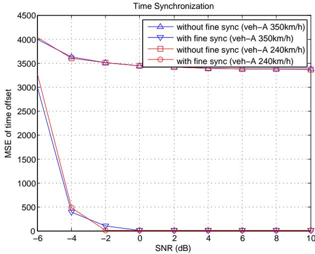
Figure 3. Mean Squared Error of time synchronization
