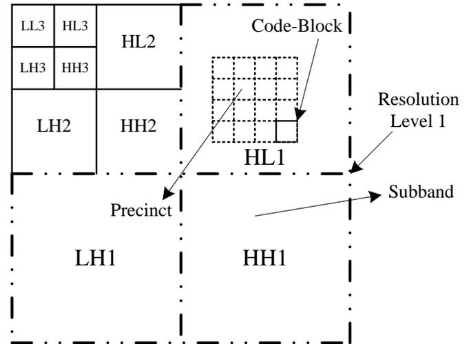
Fig. 1: Components of a JPEG2000 transformed image
