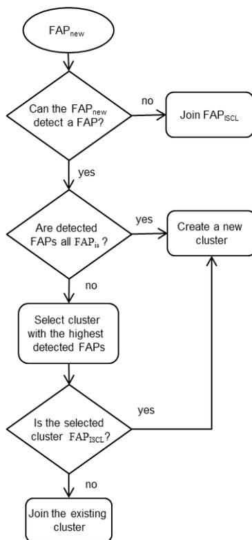
Figure 7. Steps when introducing a new FAP within a macrocell.
