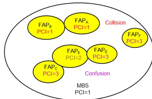
Figure 1. Example of collision and confusion events in a macrocell.
