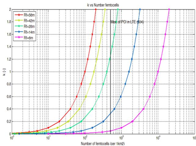
Figure 4. Number of femtocell for various femtocell radius ( $R_f$ ),  $R_m = 564m$ .
