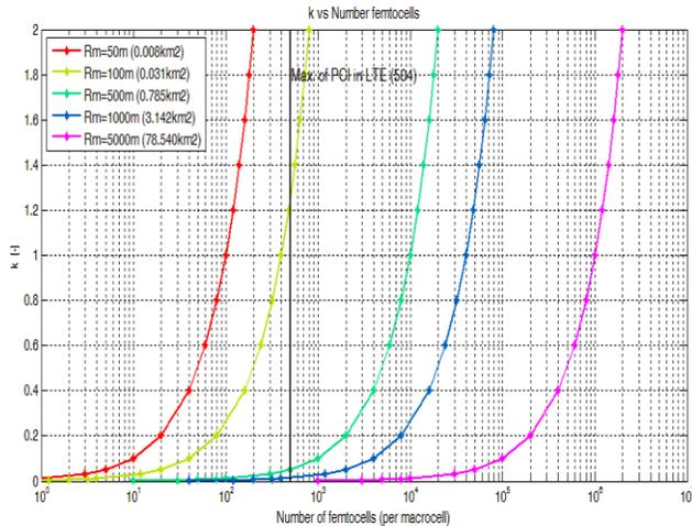
Figure 3. Number of femtocells for various macrocell radius ( $R_m$ ),  $R_f = 5m$ .
