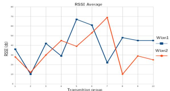
Figure 7. RSSI measured on the Mobile of WLAN1 and WLAN2
