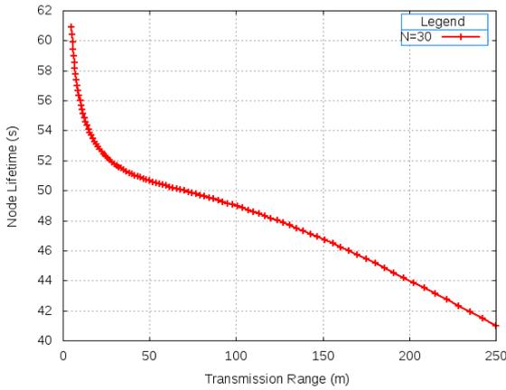
Figure 7. Node lifetime with varying transmission ranges
