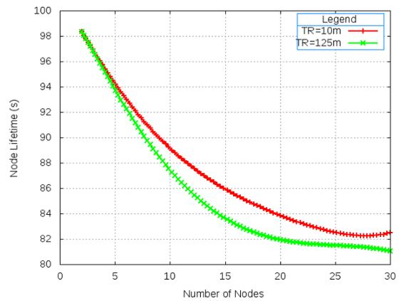
Figure 5. Node lifetime with varying number of nodes in the network
